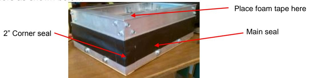
12. As in step 4, place the remaining neoprene foam tape on the top surface of the CPR to ensure a good seal between the unit and the isolation rail.
