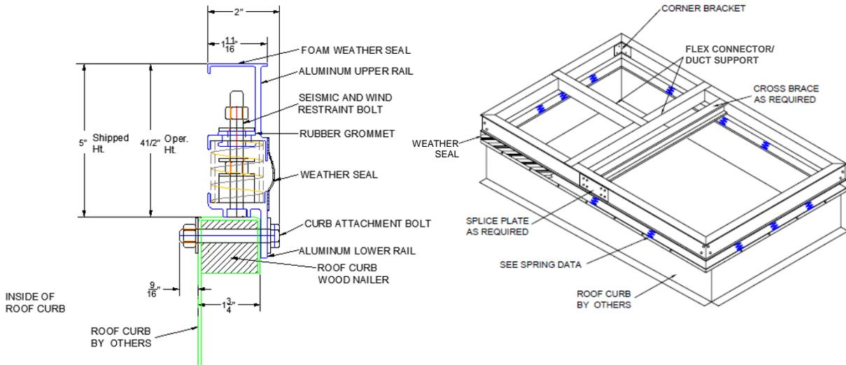
supplied  $\frac{3}{4}$ " wide neoprene foam tape. This tape is used to ensure a good seal between the curb and the isolation rail.
